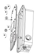
$4. \, \mbox{Install}$  the middle plate on the bottom shell and fasten it with the reserved screws.
