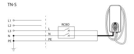
Note: RCBO is mandatory. The three-phase AC charger is additionally connected to L1 and L2.
