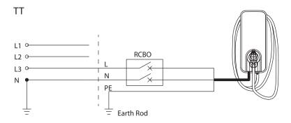
Note: RCBO and earth rod are mandatory. The three-phase AC charger is additionally connected to L1 and L2.
