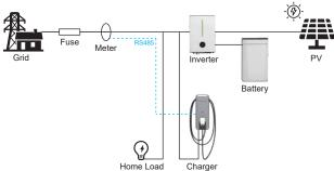
In this mode, the vehicle will be charged at dynamic maximum charging power. The charging power is continuously adjusted in response to changes in generation or power being consumed elsewhere in the home.
