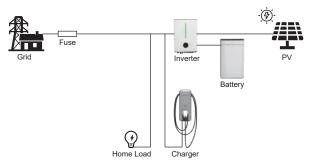
In this mode, the vehicle will be charged at fixed restricted charging power. This power can come from a renewable energy source or simply from the grid.
