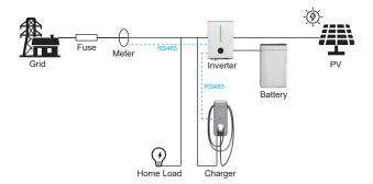
In this mode, it is a mixture of green energy and energy imported from the grid and LIVOLTEK battery pack. ECO mode minimises the use of grid power and can charge using 100% green energy.
