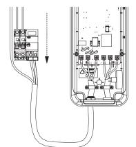
3. One 40A RCBO (type A / 30mA) must be forcibly connected to the front end of the incoming line of the charger, and the corresponding wiring shall be subject to the requirements of the circuit breaker.
