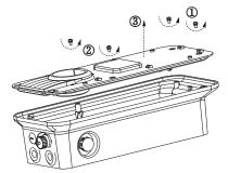
5. Loosen the 4 screws on the middle plate and open the middle plate.
