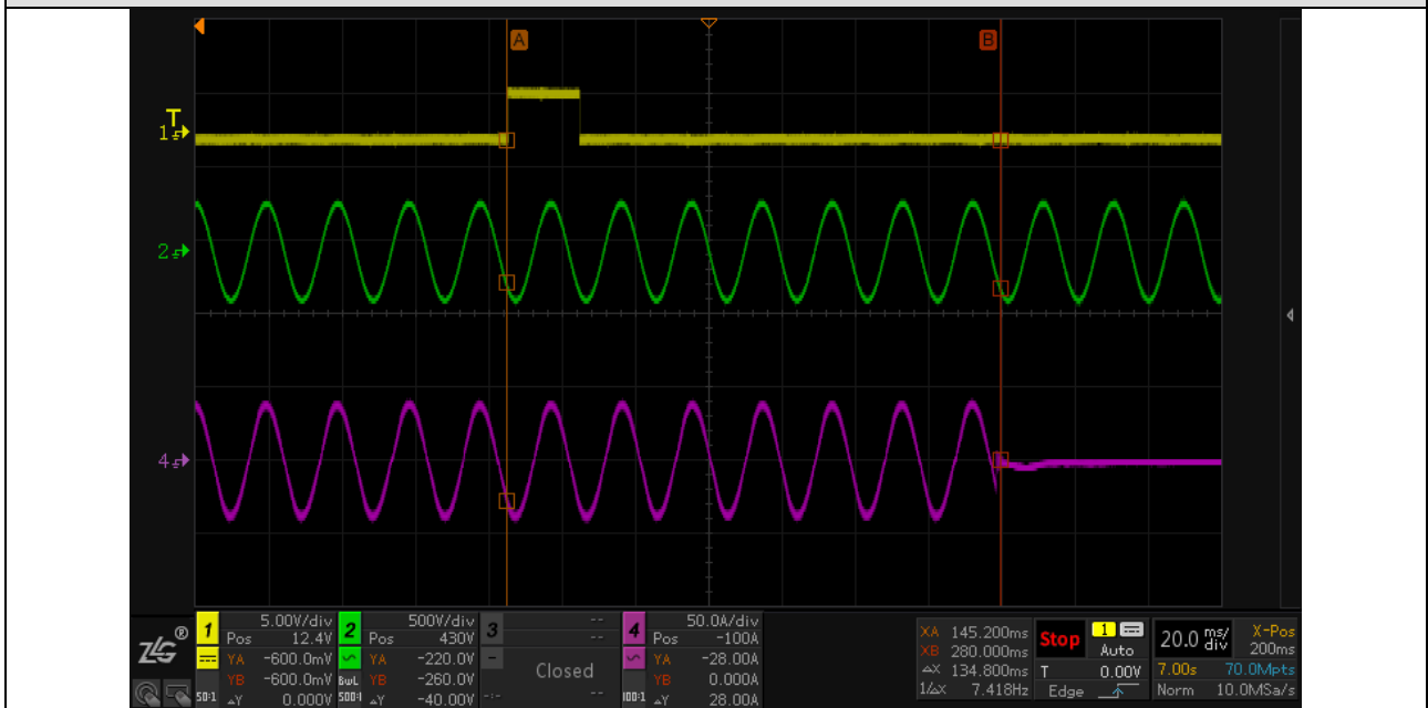
Graph of disconnection at F > (81 >)
