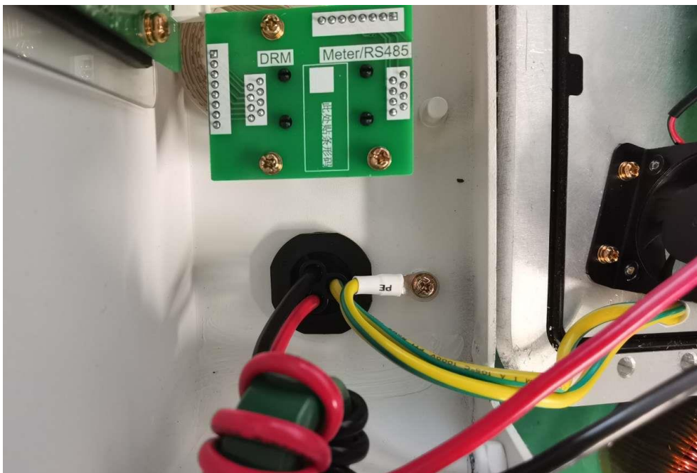
protective earth terminal GT1-3K3S1
